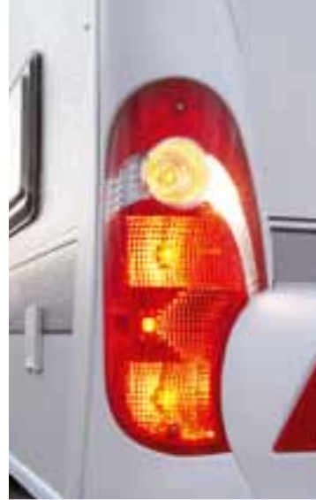
Rear lights with integrated fog lights
