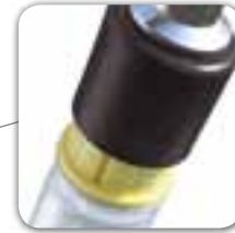
Integrated trailer nose weight display for jockey wheel (model-specific)
