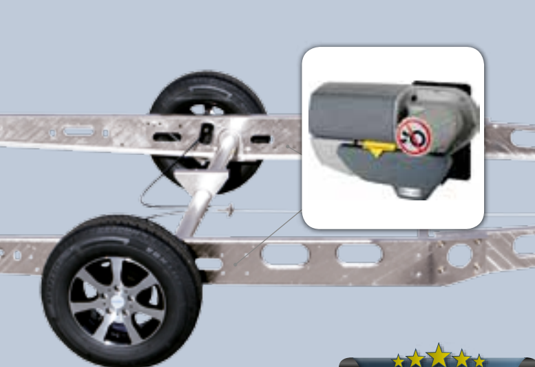
A torsion bar spring axle with longitudinal member technology including mounting fixture for TRUMA Mover
