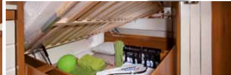
Pneumatic bed stowaway mechanism (model-specific)
