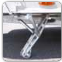
Wind-down legs (image shows heavy-load support)
